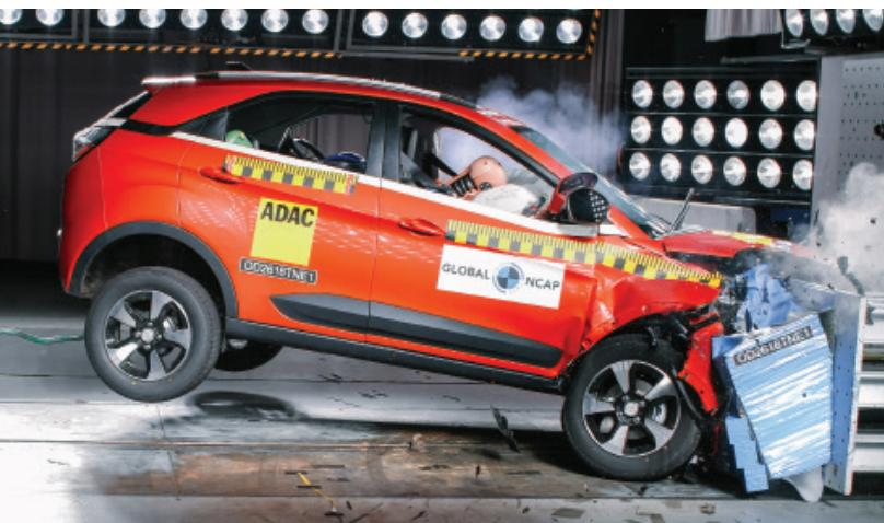
The moment of truth during the 2018 Global NCAP crash test of Tata Motors' new Nexon. The compact SUV achieved a four-star adult occupant rating and a three-star child occupant rating.
