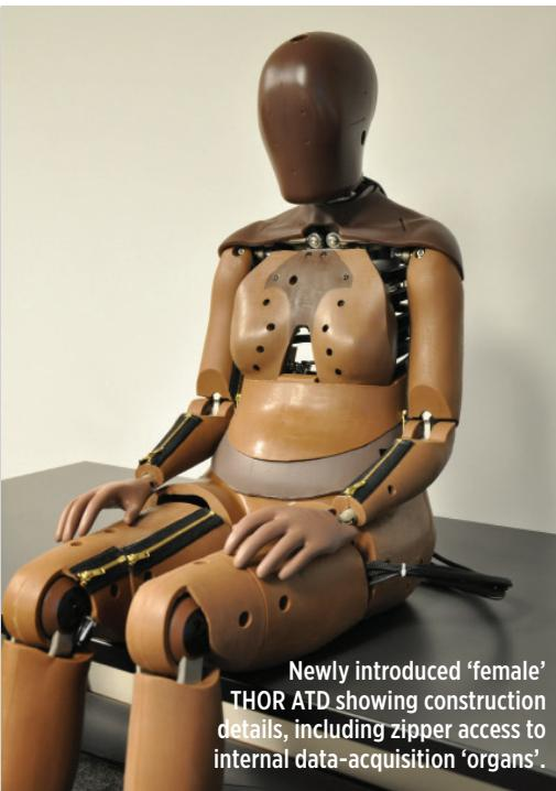
Newly introduced 'female' THOR ATD showing construction details, including zipper access to internal data-acquisition 'organs'.
