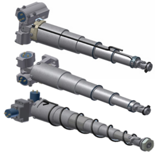
Figure 1: Three of the six varieties of devices used in THOR, upper thorax, lower thorax and abdomen, all right hand shown.
